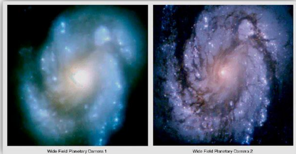
Before and after! An error in the grinding of Hubble's mirror caused it to produce fuzzy images like that of galaxy M100, left. After the addition of a corrective lens, in 1993, Hubble's image of the same galaxy became as clear as promised. Photo: NASA and STScI
